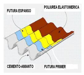
A1 Asbestos-containing materials: encapsulation (type A: external view)
